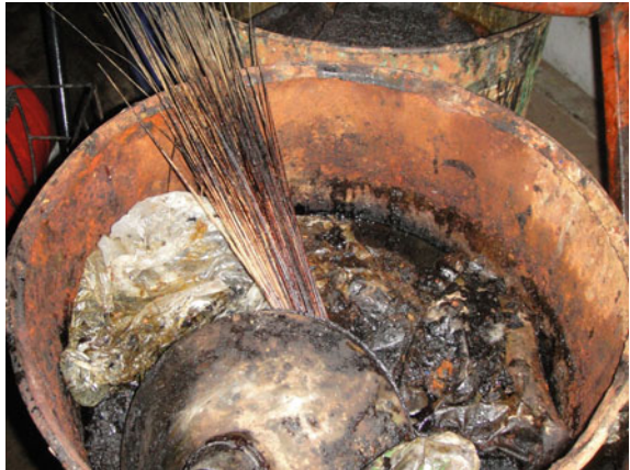
Fig. 13.16 Partially damaged raw material in a chemical industry during a fire accident
