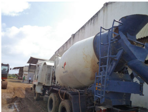
Fig. 7.11 Vehicle mounted mixer at a TSDF facility for mixing stabilisers
